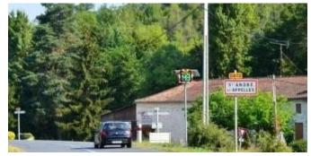
Speed is detected by a Doppler radar located inside the speed sign casing. The radar sends radar waves, the frequency of the waves reflected by the vehicle allows to calculate precisely its speed.
