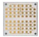
The Doppler antenna is the key element of a radar speed sign.
