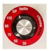
To simplify installation and avoid any computer setup, Evolis radar sign provides pre-set parameters with related to different types of speed limits in force (limited to 30 km / h areas, 50 km / h.). When installing or changing location, just turn the dial to select the correct settings corresponding to speed limit.
